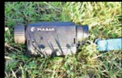
A modern thermal imaging device used to detect heat sources (wild animals).
