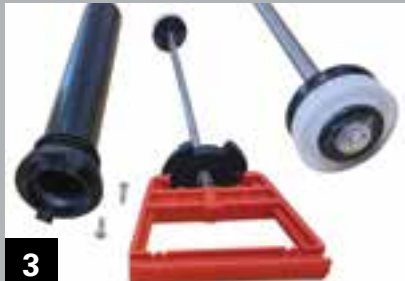
3 The internal washer is also vital – this pushes air through the pump which then passes through the valve to build the pressure. Rarely does this washer fail, but it is not uncommon for them to lose efficiency. The application of a small amount of Vaseline or WD40 around this washer will ensure a smooth action through the pump mechanism.
